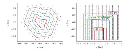
Active volume decreases with deposited energy — threshold reduced to  $\sim 1\,\text{TeV}$
