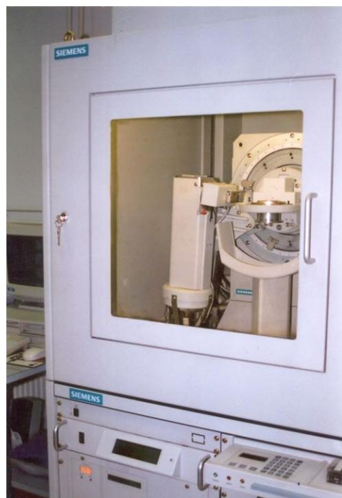
Slika 19: Rentgenski praškovni difraktometer Siemens D5000 (Rentgenski, 2009)
