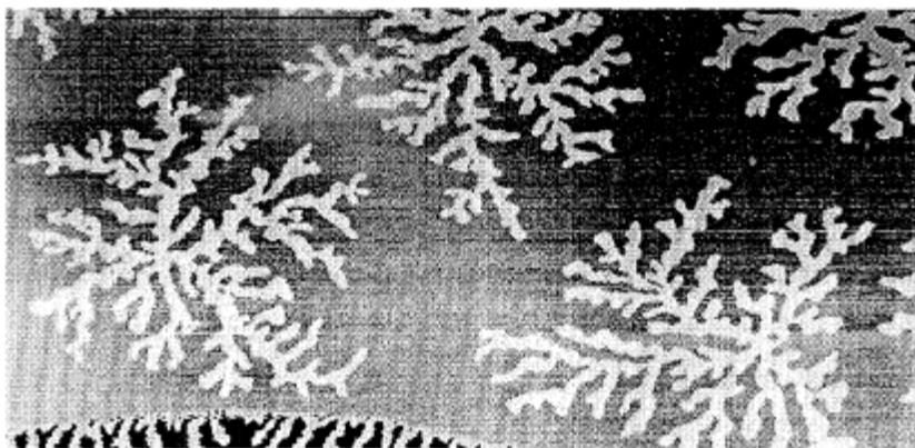
Fig. 3.3: STM image of Au islands on Ru(0001). Image size is 1.00\mu\text{m} \times 0.65\mu\text{m} . Figure has been taken from Ref. [100].
