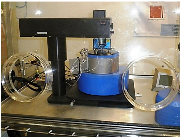
Fig. 2.11: Commercial Veeco CP-II AFM used in our laboratory
