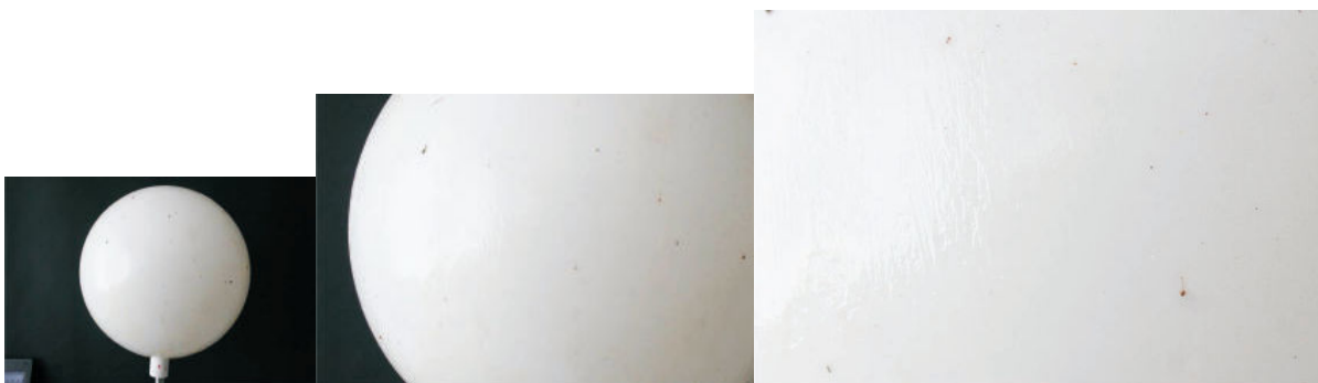
Figures 150, 151 and 152: Collected particles on the surface of a sampler oriented away from Port of Koper and EET depot
