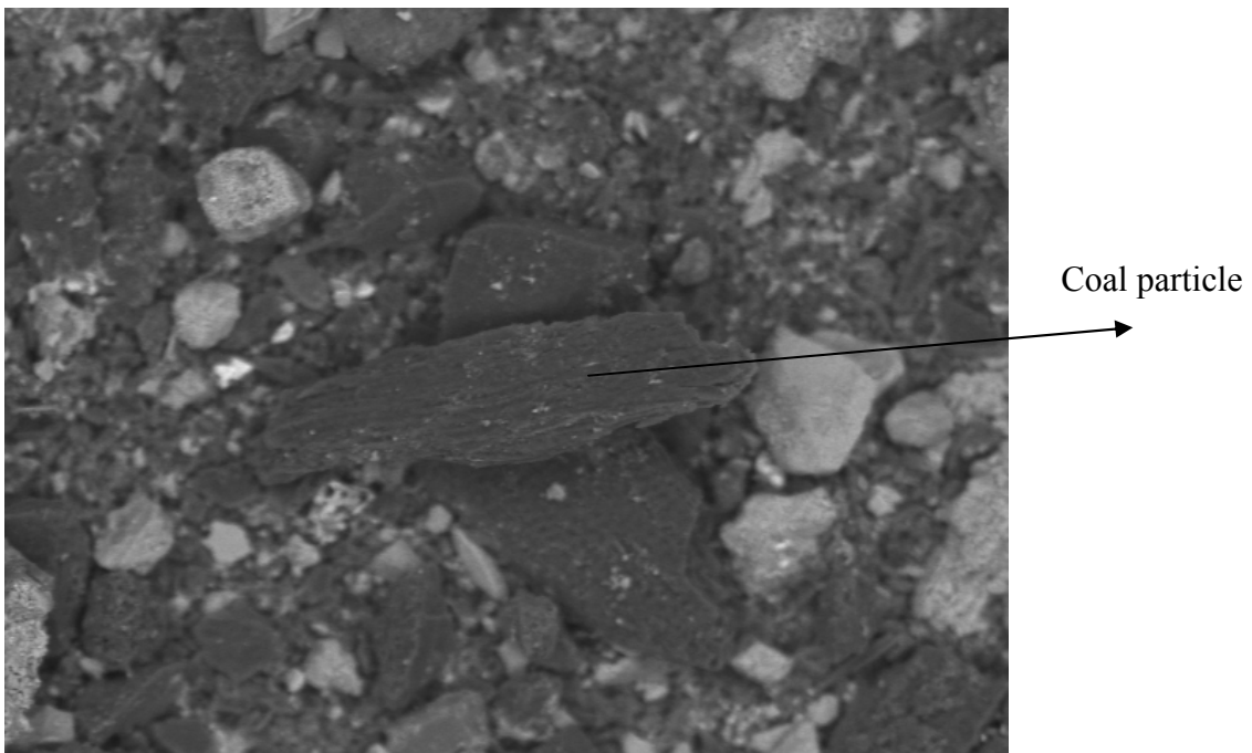
Figure 75: Sample 4A (220x magnification, image width 600 \mu\text{m} )
