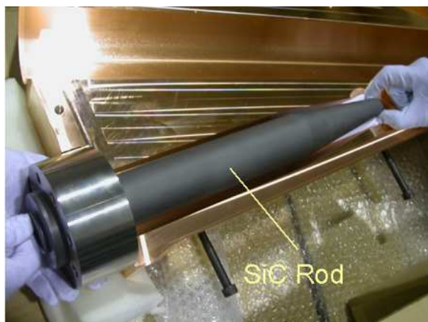
Figure 9.27: SiC rod in a winged HOM damper.
