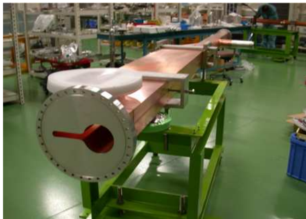
Figure 9.24: Prototype ante-chamber (1st trial model).
