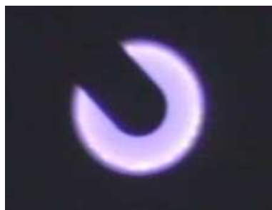
Figure 8.14: Multipactoring discharge in bright blue inside the coaxial line of the input coupler, observed with a TV camera from the opposite side of the driving port. The silhouette of the coupling loop can be seen at 10 o'clock.
