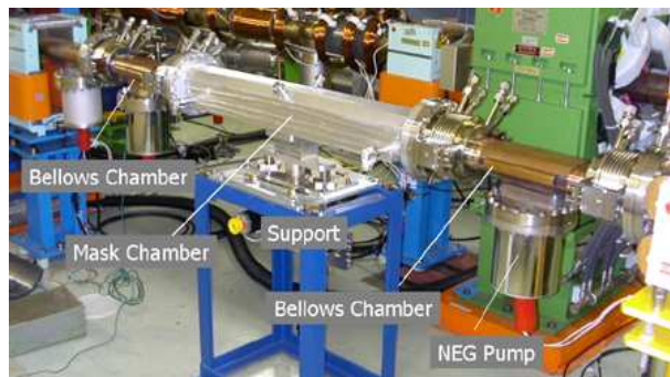
Figure 9.15: Mask chamber (vertical) in the present KEKB HER.
