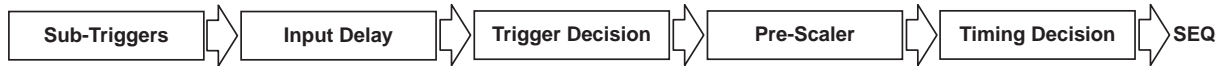
Figure 3.71: Schematic view of Global Decision Logic(GDL) stages. The final output from GDL is sent to SEQ.
