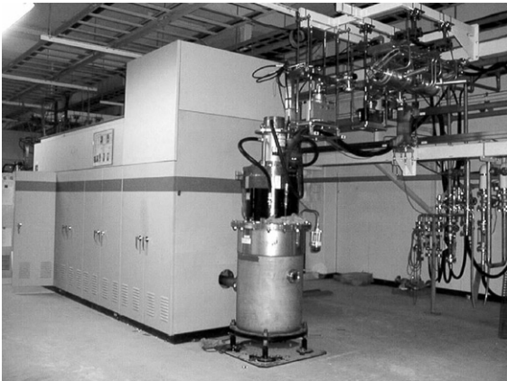
Fig. 10. The entire picture of the modulator, the klystron assembly and the SLED cavity.
