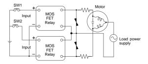
Operate SW1 for at least 30 ms after SW2 has been operated, or vice versa.
