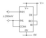
Measuring an input voltage referenced to a floating supply, i.e. the input voltage and the meter's power supply are isolated from each other.
