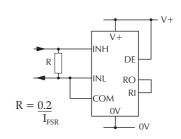
Measuring current. The meter's supply is isolated from the current being measured.
