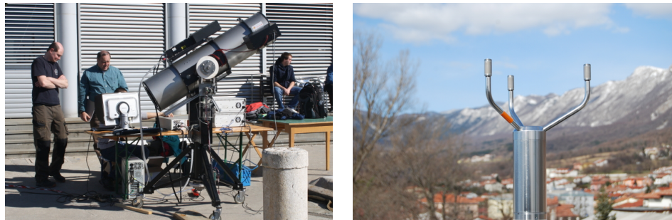
Figure 1: Mie-scattering lidar system of University of Nova Gorica (left) and ultrasonic anemometer, positioned at the rooftop in Ajdovščina (right).
