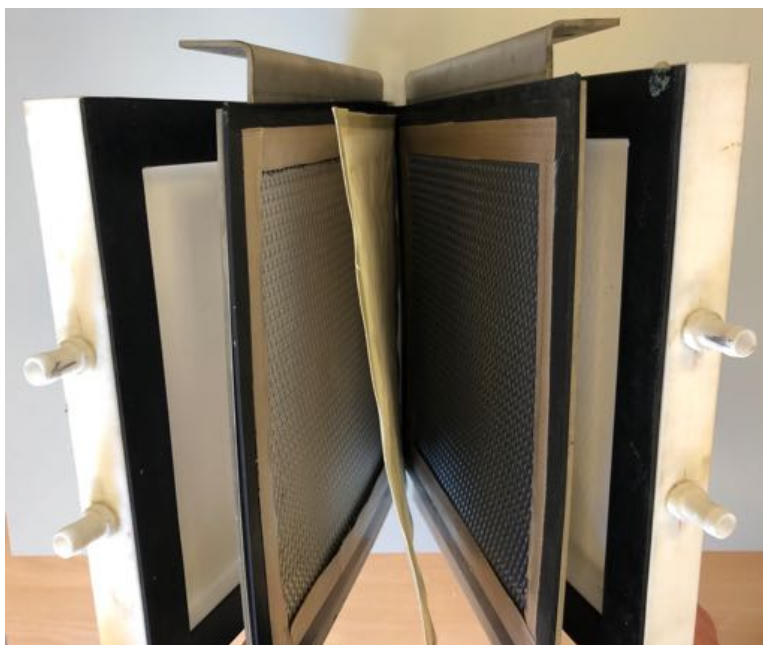
Figure 5: Expanded view showing the components of the electrolytic cell. The two white half-cell parts on the sides are made from PTFE. The black parts are four EPDM rubber gaskets of which two are placed in-between each half cell and electrode, the remaining two are placed in-between each electrode and membrane with visible additional brownish masking tape towards membrane. Two electrodes of which cathode is the left light gray anode is the right dark gray. In the middle the light yellow is the anion exchange membrane AMI7001s (Membrane International, USA).
