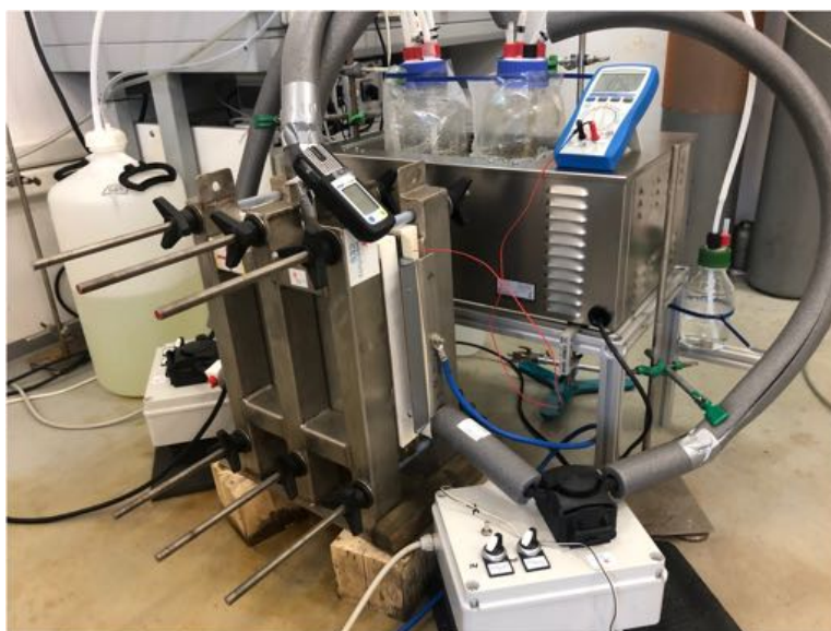
Figure 4: The constructed experimental electrolysis system with visible parts. Inside oil bath are two boro-silicate glass tanks with blue multi-connection caps, single a electrolytic cell mounted into dedicated press and two peristaltic pumps on the sides.
