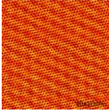
Figure 10: The high resolution STM image demonstrates the cleanliness and flat surface of graphene supported on MoS_2 . The graphene honeycomb lattice is noticeable, along with a faint moiré periodicity apparent only at very high tunneling current ( I_t = 33 nA and V_{bias} = -50 mV). Image adopted from [21].
