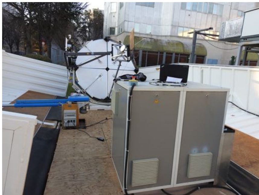
Figure 4: Barcelona Raman LIDAR in opened container at its site in Universitat Autònoma de Barcelona, Spain. The blue piston is one of actuators holding container halves in opened position.
