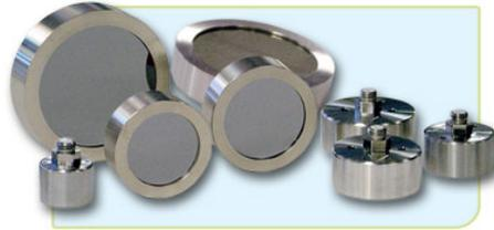
Figure 13: A range of ion–implanted diode detectors in metal casings. The front side has a circular opening of slightly darker colour, called the detector active area [9].
