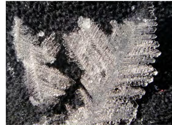
experimental observation: dendrite tip = paraboloid of revolution
